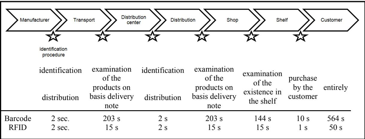
Figure 3. Cost reduction potential of RFID [7].
